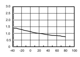
Fig.6 Relative Radiant Power vs. Temperature
