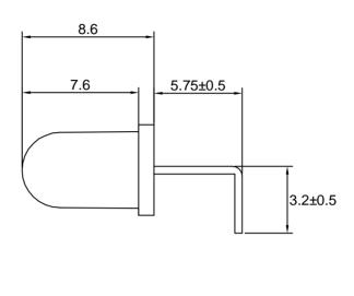
Note: 1.All dimension are in millimeter tolerance is ±0.25mm unless otherwise noted.
