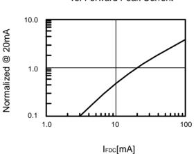
Fig.4 Relative Radiant Power vs. Forward Peak Current
