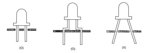
The LED lamps are designed for high-density mounting and have a structure which can alleviate mechanical stress due to clinching. Nevertheless, take care to avoid the occurrence of residual mechanical stress due to clinching.
